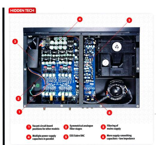
DAC chip and the circuits around it have some very serious jitter-reduction measures built in and, short of jitter so bad it causes stuttering (which would imply a seriously broken source), that particular bogey seems to have been rendered harmless.
