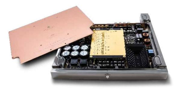
It's effectively added 50% more power to the previous models, and includes more filter inductors per channel. The analogue to digital conversion stage (Magic Wire in Devialet-speak) is new, too, knocking 6dB off the THD and cutting the noise floor by 2.5dB. Add in a power supply that can now deliver 4kW and a very sophisticated (and large) thermal management system, which includes a 2.5kg copper base plate, and it all becomes clear that this is not simply old wine in new bottles.
