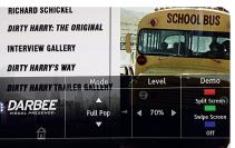
→ The Darbee interface pops up when you press the button on the Oppo's handset – cursor keys are then used to switch between modes and increase or decrease the strength of the processing
