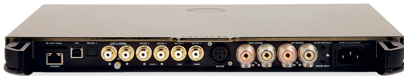
ABOVE: Three sets of RCA sockets are configurable as digital ins or line/phone analogue ins. Other digital ins include USB, ethernet (RJ45), AES/EBU (XLR), optical (Toslink and 3.5mm jack). Single sets of 4mm speaker cable binding posts are included alongside SD card (setup) and triggers (3.5mm jacks)
