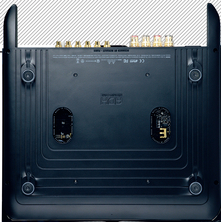
ABOVE: The underside of the 170 is an alloy injection-moulding with apertures for the (ZigBee) Wi-Fi antenna. Though still 'square' the case is about ½in smaller than the original D-Premier
