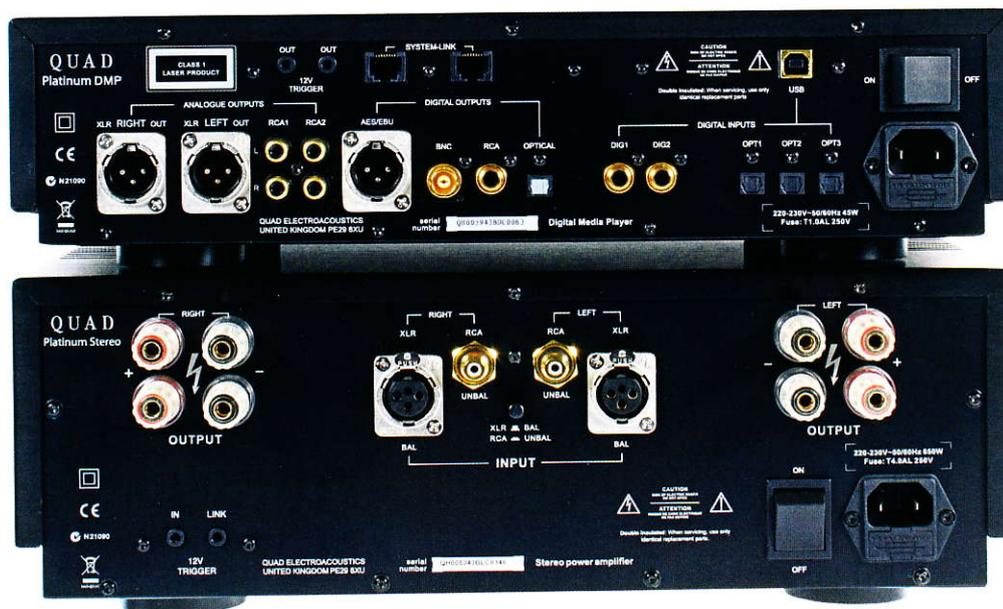
*The Platinum Digital Media player (top) has a wide array of digital inputs on its back panel, including professional AES/EBU balanced S/PDIF digital. Together with a CD player and USB, it caters for most digital audio sources. It outputs analogue to the Platinum Stereo power amp (below) through normal phono cables, or fully balanced XLR cables.*
