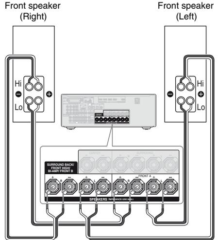
Connect the jacks on the Lo (or Hi) side of the front speakers to the SPEAKERS FRONT A terminals, and connect the jacks on the Hi (or Lo) side of the front speakers to the SPEAKERS SURROUND BACK/FRONT HIGH/BI-AMP/FRONT B terminals.
