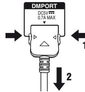
Press and hold both sides of the connector and then pull out the connector.
