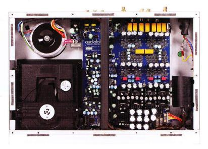
ultra low noise discrete designs, combined with LC filtering for maximal interstage and RF isolation; a total of almost 250,00uF of bulk storage capacitance is used within the CDQ. Each section of the player is independently regulated, Audiolab says.
